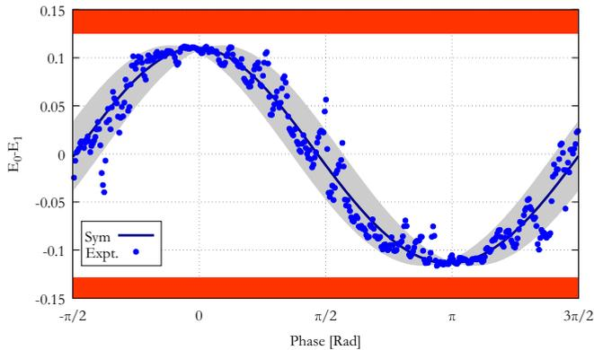
FIG. 4. Correlation function with respect to the phase difference between the two arms of the interferometer. The solid line corresponds to the simulated behavior of the device without phase fluctuation. The gray area corresponds to a relative phase uncertainty region of  $\pm 10\%$ . The red (dark) area corresponds to the region of correlations unachievable once the bound on the energy  $\omega$  is chosen to be 0.0025.
