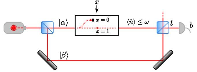
FIG. 1. Self-testing quantum random-number generation based on bounded energy. A signal coherent state is modulated depending on the input  $x$ . The signal is blocked for  $x = 0$  and transmitted for  $x = 1$  and the average energy after the modulation is bounded by  $\omega$ . The signal is mixed with a local oscillator on a beam splitter with transmittivity  $t^2$  and measured by a single-photon detector.
