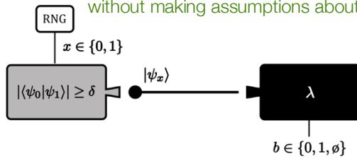
This approach provides a practical solution for semi-DI QRNG allowing some, easily verifiable, assumptions, significantly simplifying the schemes.
